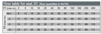
It is recommended to design for operation at a maximum of 70% of the flow values. If the diaphragm is designed in M / HC, the flow is reduced by 50 %.
