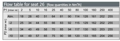
It is recommended to design for operation at a maximum of 70% of the flow values. P1 = regulating pressure
