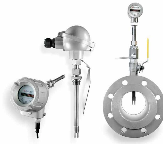
Each flow meter will be tested prior to shipment and calibrated at our CAMASS® Calibration Lab under actual operating conditions (piping layout, gas composition, pipe diameter, flow direction...). The sensor uses the thermal dispersion principle and directly measures in dry gases the gas mass or volumetric flow at standard pressure and standard temperature (according to DIN 1343: 0°C, 1,01325 bar, 0% rel. humidity). It consists of a heated electrode and a reference
