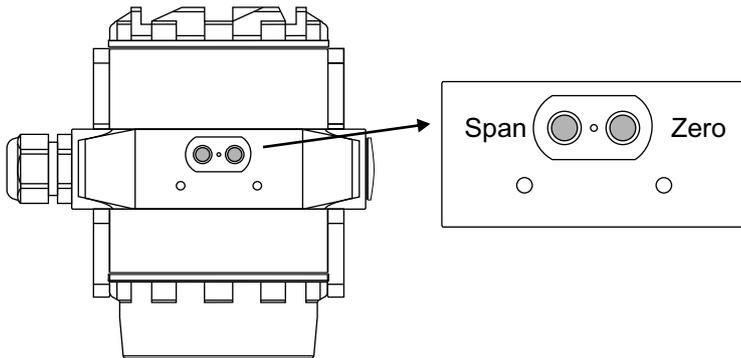
Below the type plate there are 2 key button for easy configuration of zero and span. The keys are Hall effect devices and are completely separated from other parts of the enclosure.
