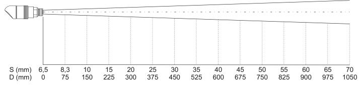
S = Spot size D = Distance from front of the sensing head to the object
