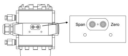
Below the type plate there are 2 key button for easy configuration of zero and span. The keys are Hall effect devices and are completely seperated from other parts of the enclosure.
