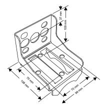
Holder made of steel (zinc coated) for mounting the device on walls or tubes is supplied with the device.
