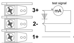
The 4...20 mA test can be measured without interruption of the low-potential circuit between terminal 3(+) and terminal 2(-). The output current is measured with an ammeter for mA across a diode in the output circuit.
